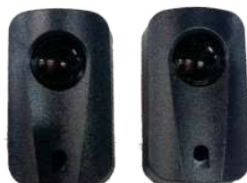
SKN-PC-11 Power supply : 12V~24V AC/DC Max. Range: 15M Input: RX 15mA, TX 30mA Infrared frequency: 1.92KH Wave length: 940nm Relay output: 1A max 36V
