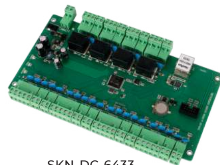
SKN-DC-6433 4 Door / 8 Reader Communication : LAN Register Cards : 42000 Record Capacity : 200000 Camera can be Integrate Input: Wiegand26/34
